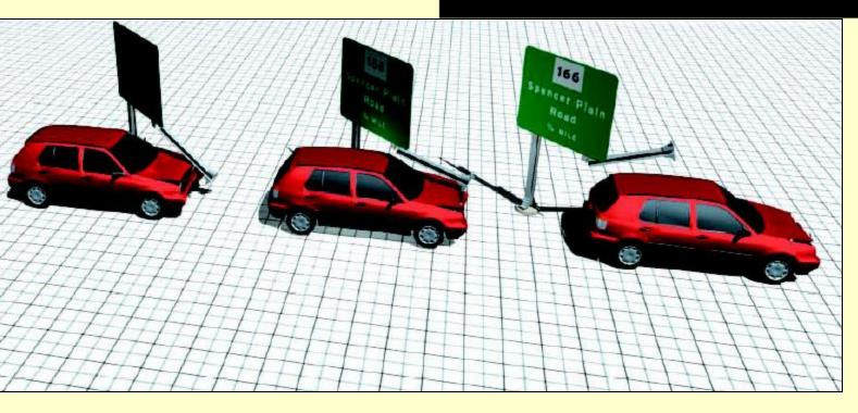
The angle of an errant vehicle leaving a highway impacting a roadside structure is impossible to predict. Most breakaway support systems are one directional in their design and crash performance.
