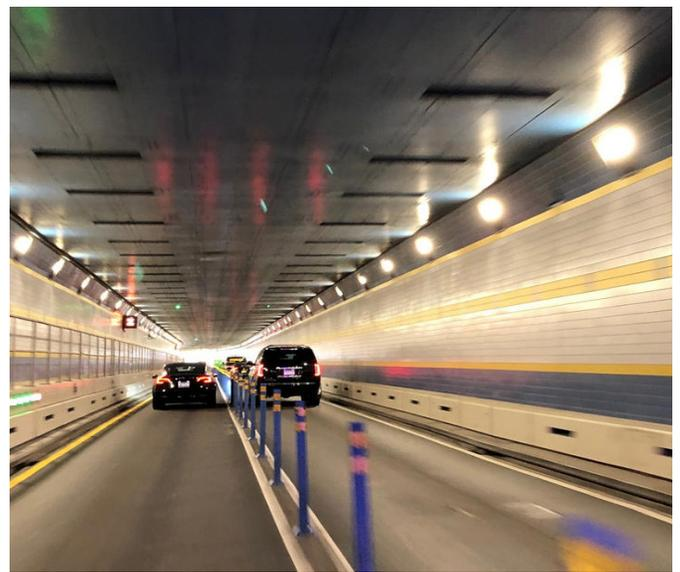
Visi-Barrier® is a high visibility panel for driver safety. A sustainable solution for new and aging tunnel bench walls, offering corrosion and impact protection
